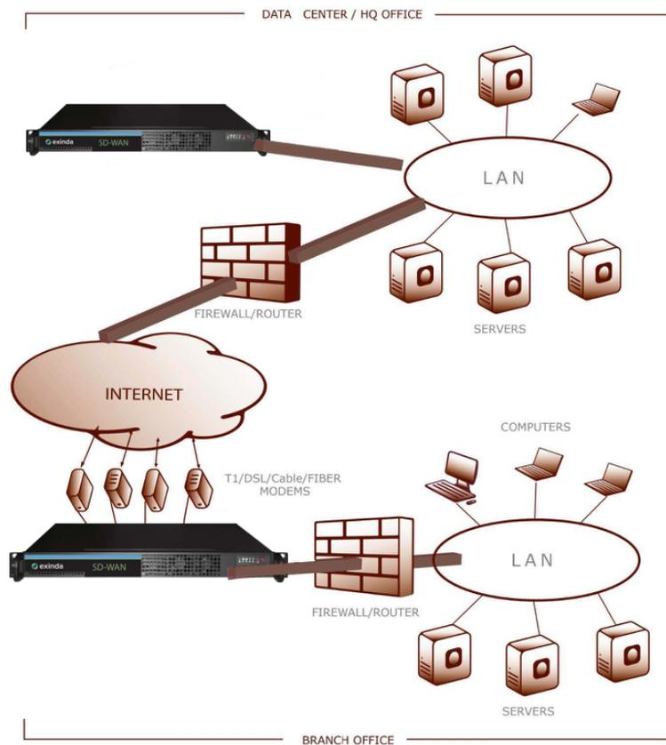
The two Exinda devices form a transparent, high-speed data tunnel between them by combining access resources on each side.
